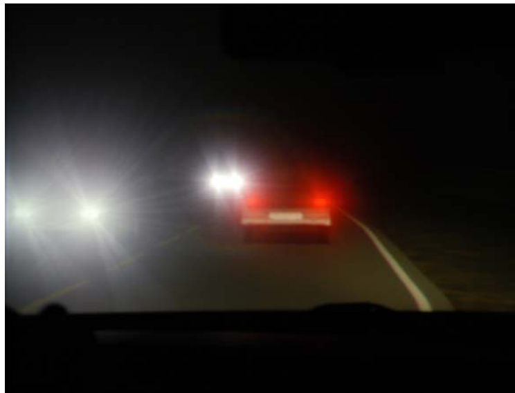
Blooming effects for incoming vehicles rendered in night conditions with SCANeR II©
